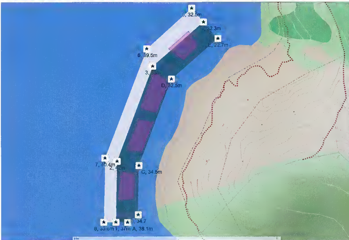
Figure 3. Depths of the proposed extension area (grey), parent farm (teal) and existing surface structures (pink).
