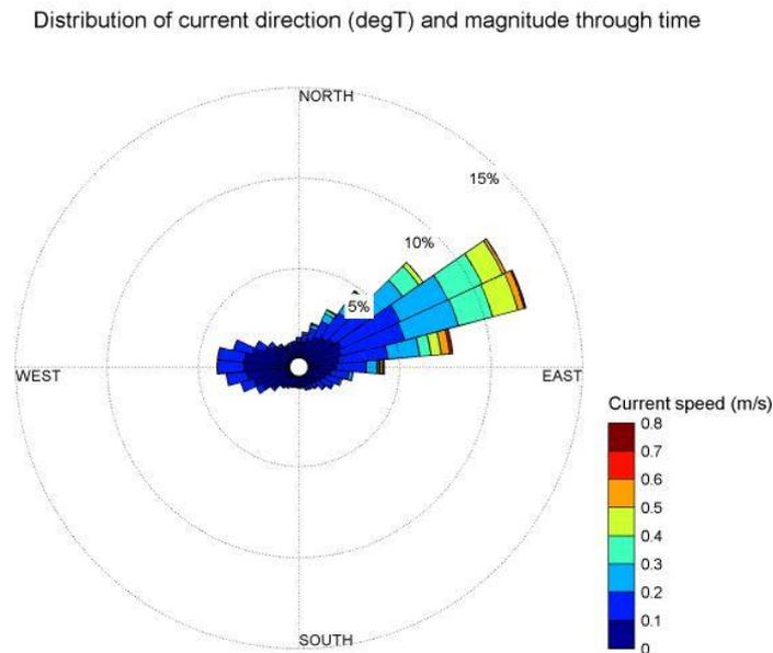
Figure 3-7: Current rose showing current directions and magnitudes for all bins at Blowhole Point South.
