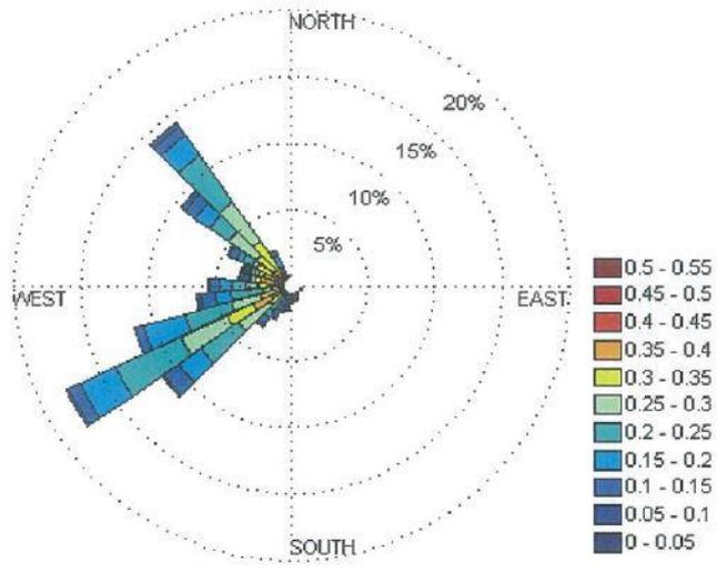
Figure 3-7: Current roses showing percentage distribution of speeds and direction at 20 m in the water column.
