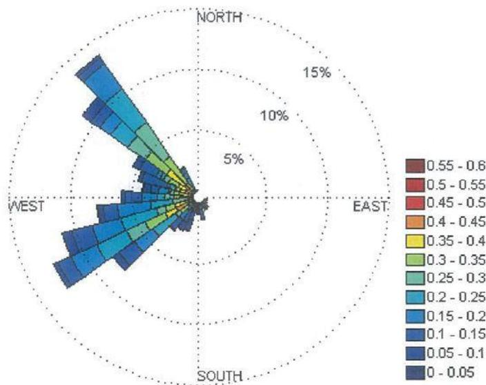
Figure 3-5: Current roses showing percentage distribution of speeds and direction at 5 m in the water column. .
