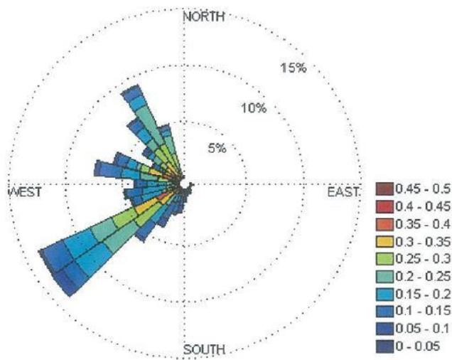
Figure 3-9: Current roses showing percentage distribution of speeds and direction at 34 m in the water column.
